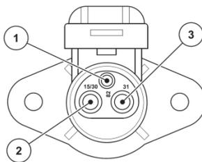
**Figure 3.1** Pin layout of the power plug socket: 1 STICK - unused, 2 STICK - (15/30) +12 V, 3 STICK - (31) ground.
