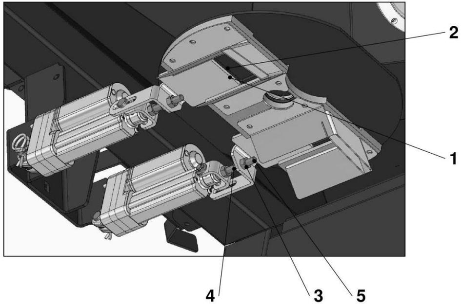
**Figure 4.10** Metering system: 1- face plane of the gate valve, 2- face plane of the hole in the bottom of the tank, 3- lock nut M8, 4- thrust nut M8, 5- adjusting screw M8.
