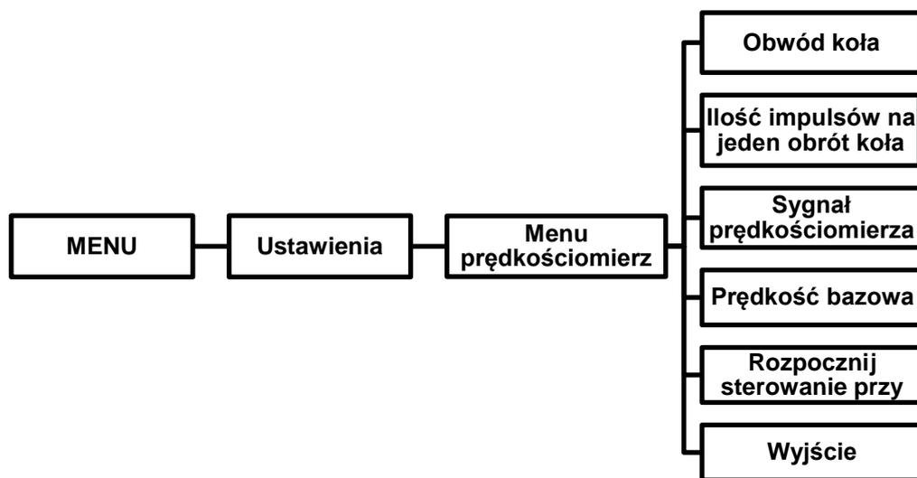
**Figure 4.5** Diagram of the speedometer menu.
