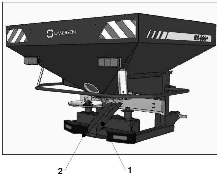
**Figure 4.9** The spreader during the calibration test: 1- island trough, 2- rear beam of spreader frame.
