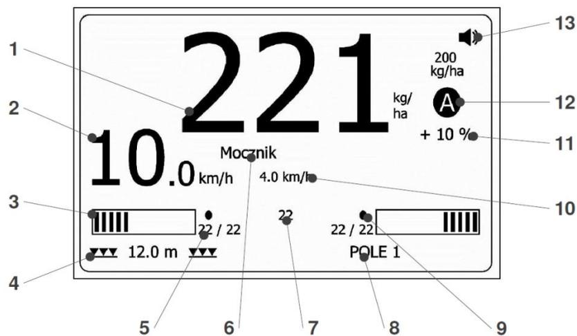
**Figure 2.4** Work screen during fertiliser spreading in automatic mode.
